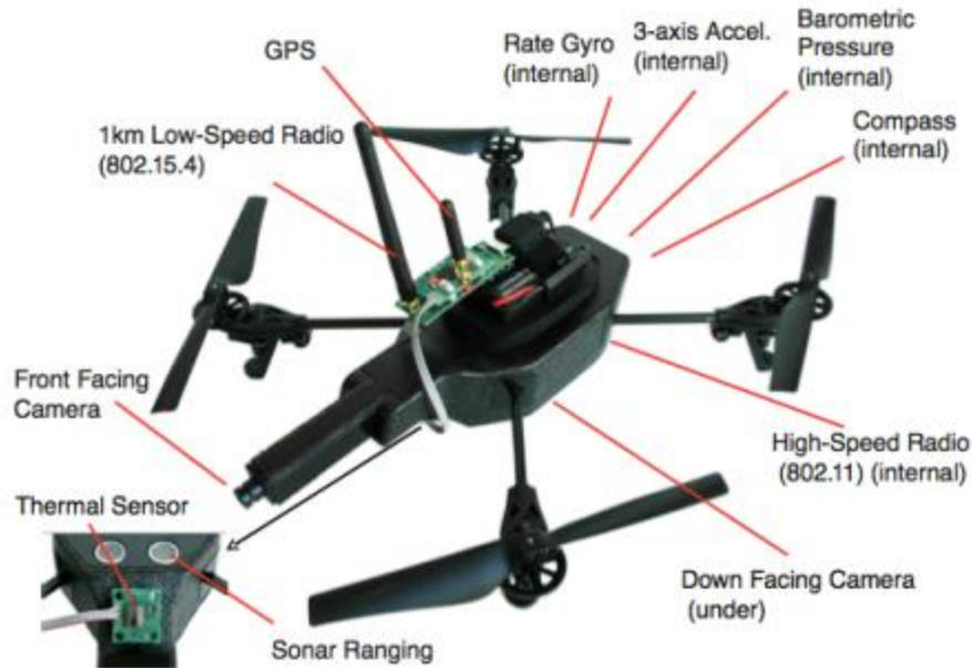
Figure 2.1 Structure of a commercial drone Source: (Rao et al., 2016)
