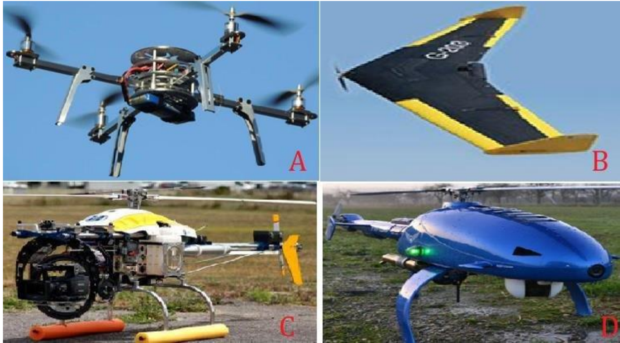
Figure 2.2: Types of drones currently in use: A (Multi Rotor), B (Fixed Wing), C (Single Rotor) and D (Hybrid). Source: CircuitsToday, 2018.
