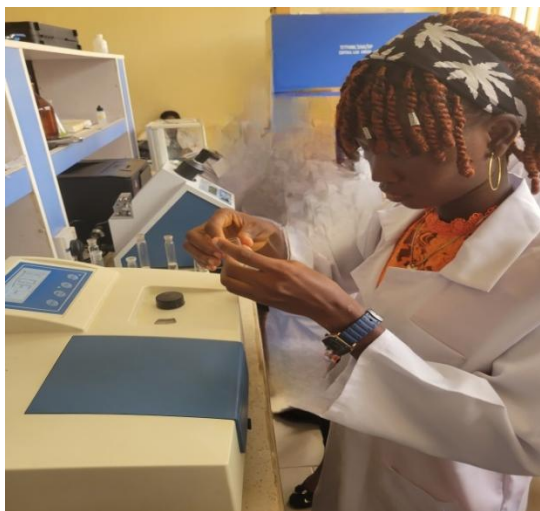
Figure 2.3: Measurement of absorbance of the standards
