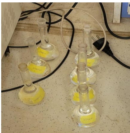
Figure 2.2: Standard Solutions of 10, 15, 20, 25, 30, 35 and 40 ppm
