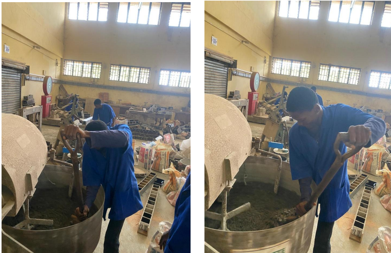
Plate 2: Casting process of concrete
