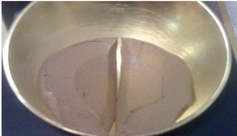
Fig 3.2 Casagrande Cup measurement of the Liquid Limit
