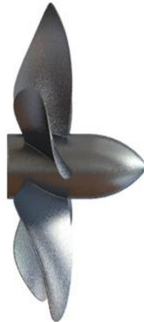
Figure 3.2: side views of the 3d model of the vp1304 propeller used in the analysis
