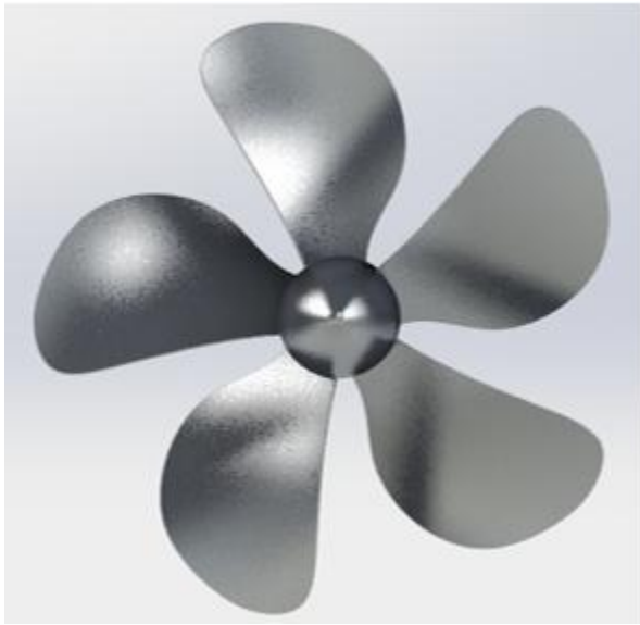
Figure 3.1: front and back view of a solidworks model of the vp1304 propeller used in the analysis
