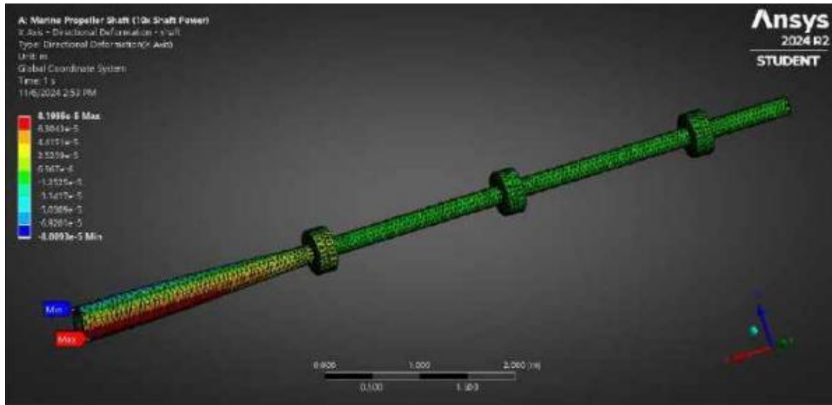
Figure 4.3: Contours of X-Axis Directional Deformation
