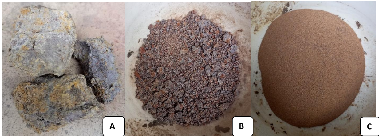
Figure 3.1 Clay sample preparation process. A) Raw clay sample. B) Crushed clay sample C) Sieved clay sample.
