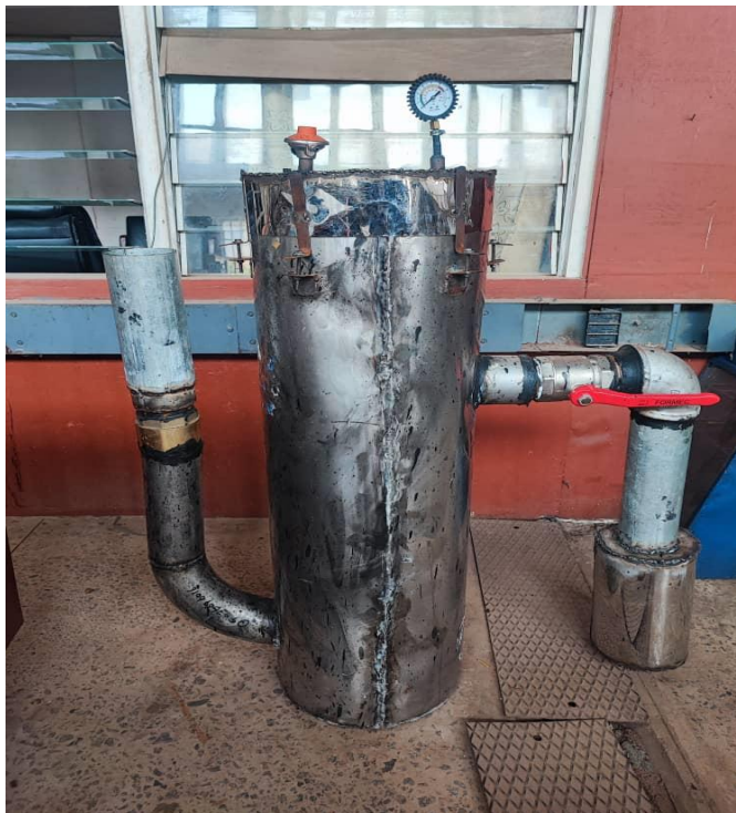
Fig. 4.1 the Biogas Digester
