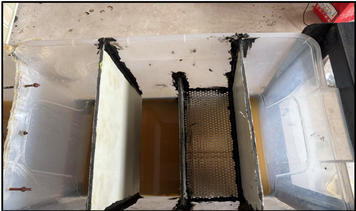
Plate 2: Greywater in the Flocculation Basin of the Facility
