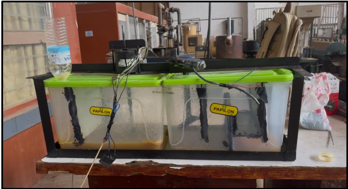
Plate 1: Coagulation-Flocculation Water Treatment Facility
