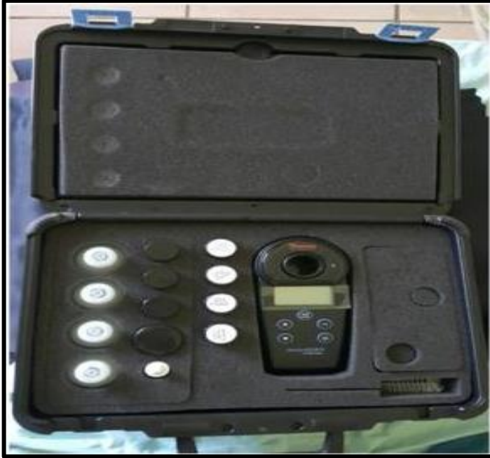
Figure 3.3: Turbidity meter (Yaka, 2018)
