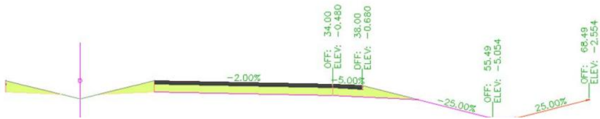
Fig 2.10: Details of the right side of the assembly used in this example.
