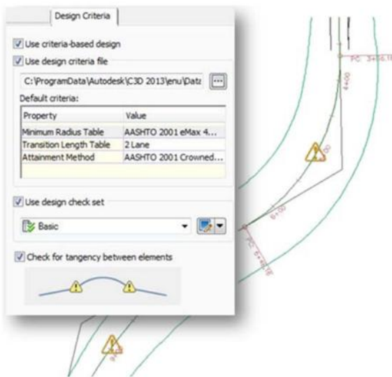
Fig 2.1: Design criteria and design check sets are options of Alignment and Profile Properties
