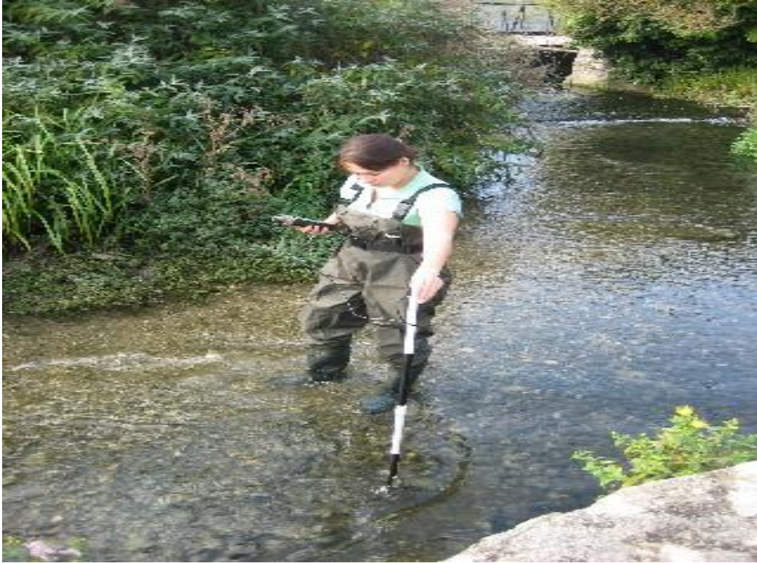
Plate 2.3: Measuring velocity of a river with a flow meter
