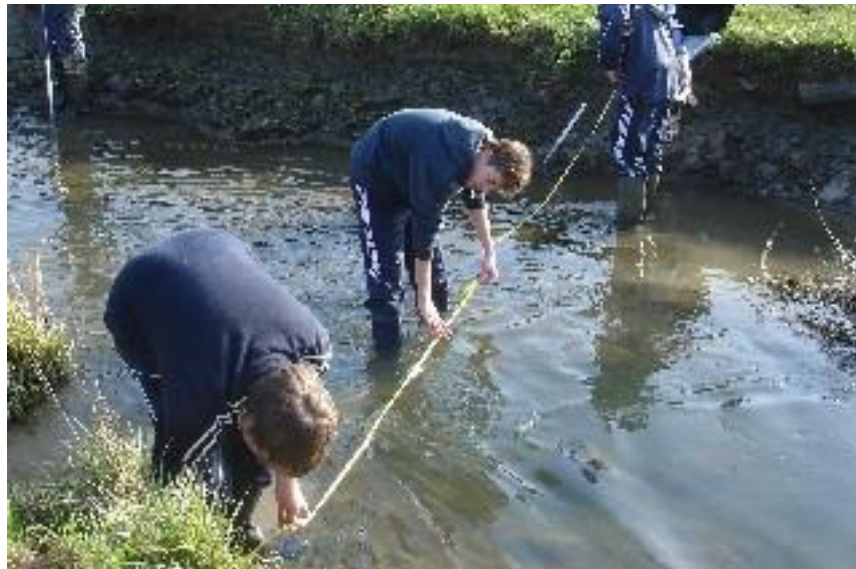
Plate 2.1: Measuring river width. ( http://water.usgs.gov/edu/streamflow3.html )
