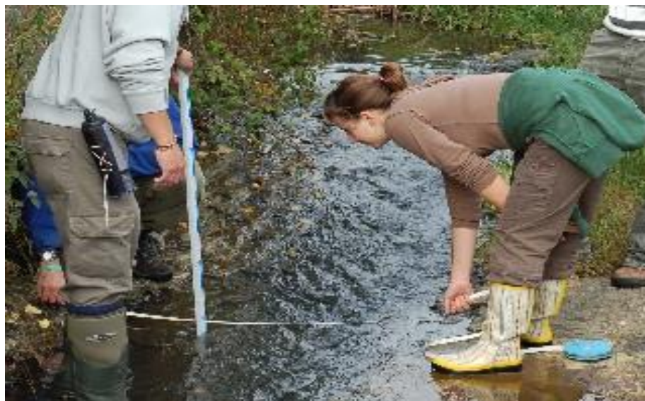
Plate 2.2: Measuring river depth. ( http://water.usgs.gov/edu/measureflow.html )
