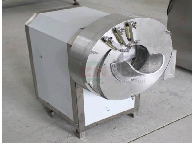
Fig 2. 9 Banana Slicer Developed by Mr. Augustin.
