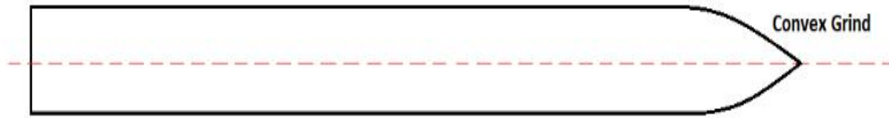
Fig 3. 6 Blade profile for convex grind (Evan Bossio et, al, 2017).
