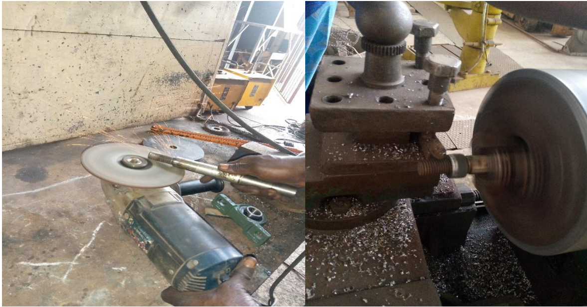
Fig 3. 29 Showing Shaft preparation
