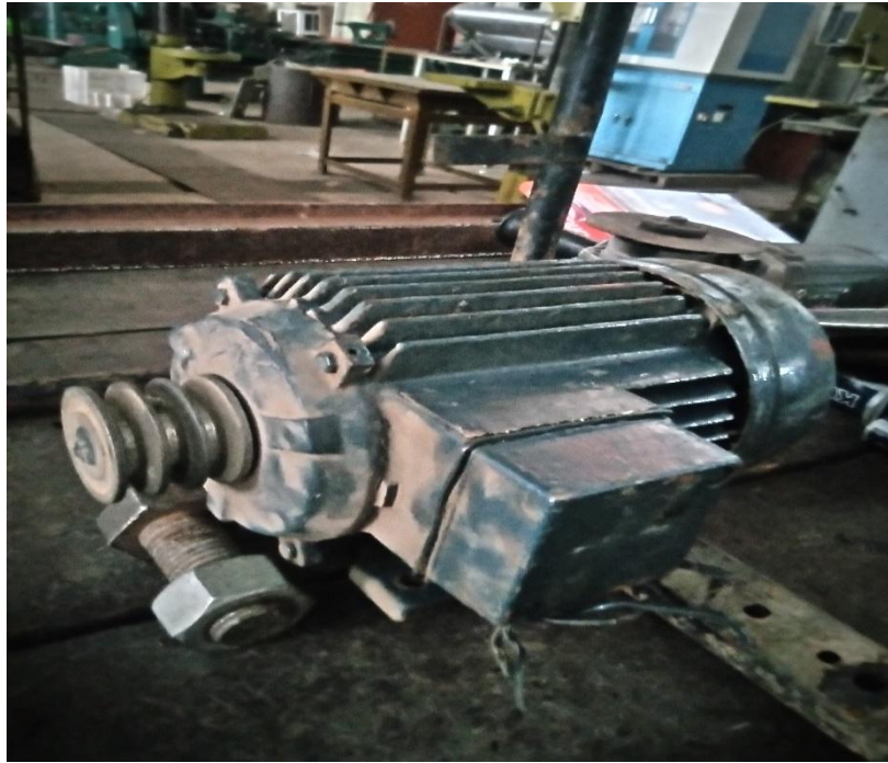
Fig 3. 35 Showing Induction motor
