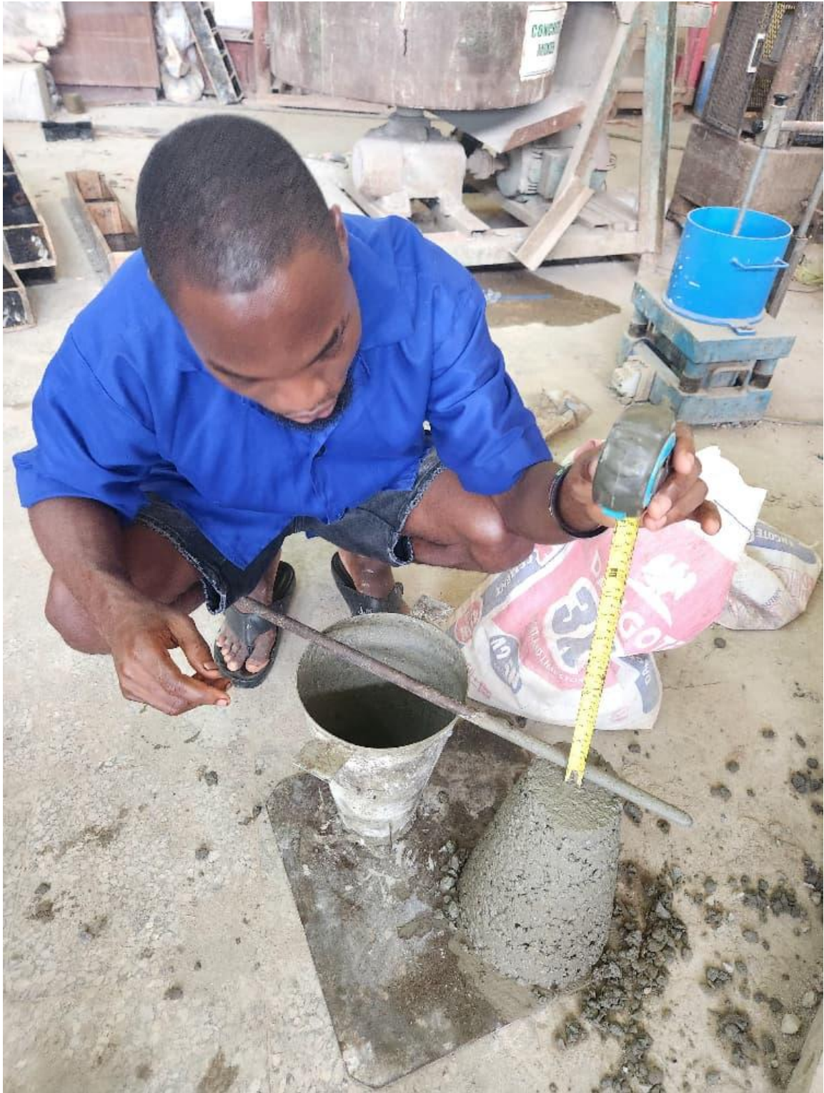
Plate C.4: Slump Test being carried out
