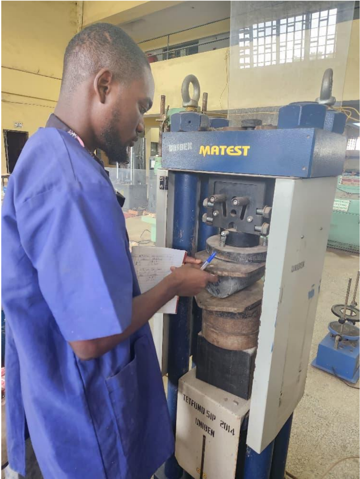
Plate C.6: Compressive Testing being carried out
