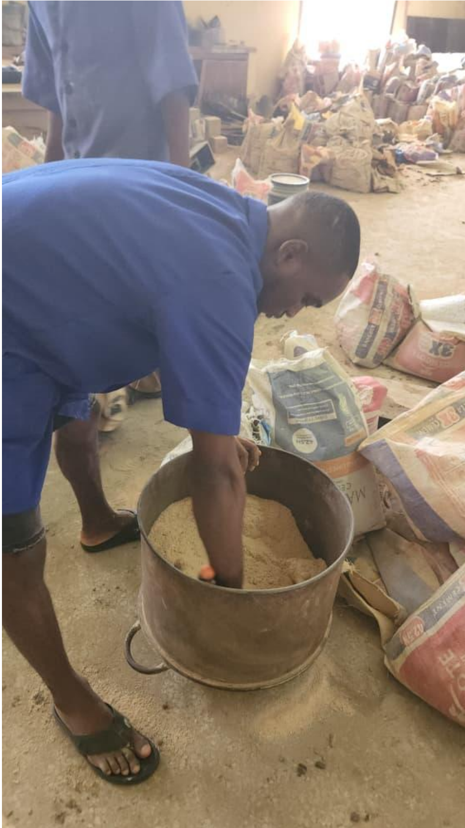
Plate C.1: Sieving of Fine Aggregate for Proper Aggregate Proportioning
