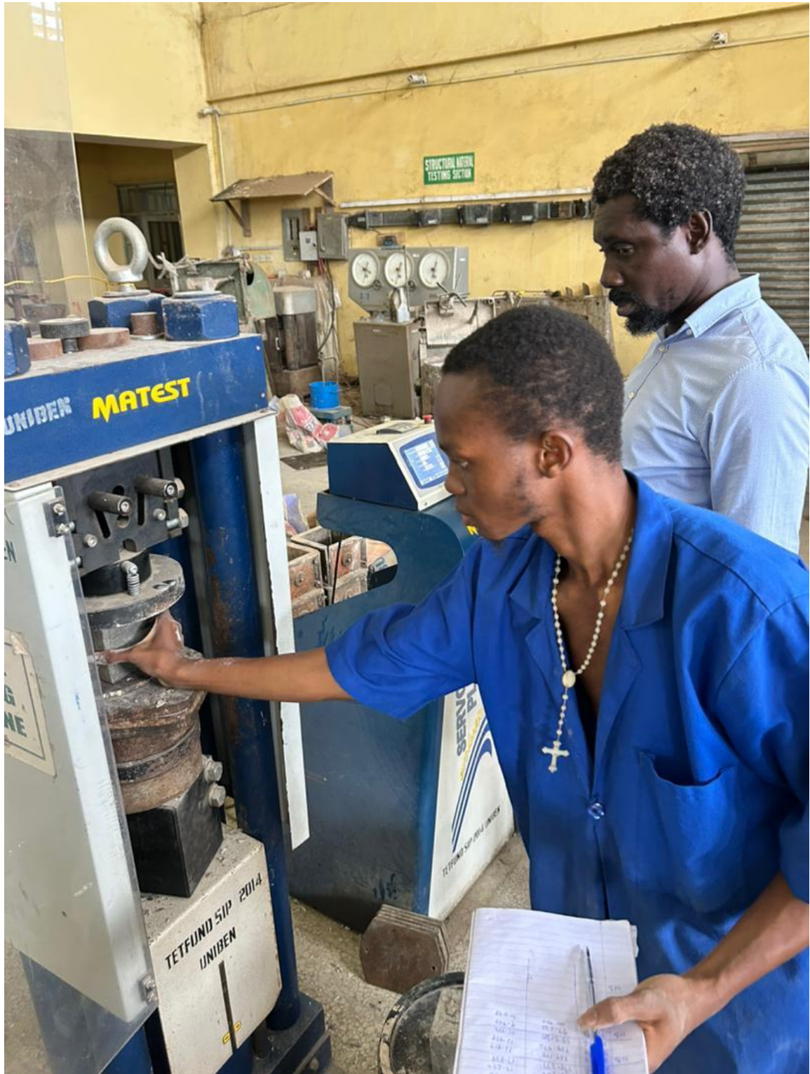
Plate 9: concrete crushing (destructive test)
