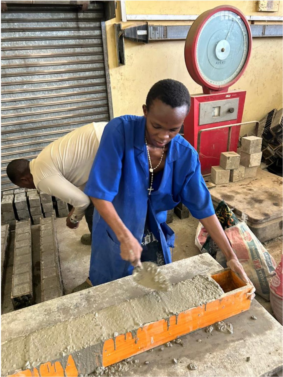
Plate 8: concrete compaction on vibrating table
