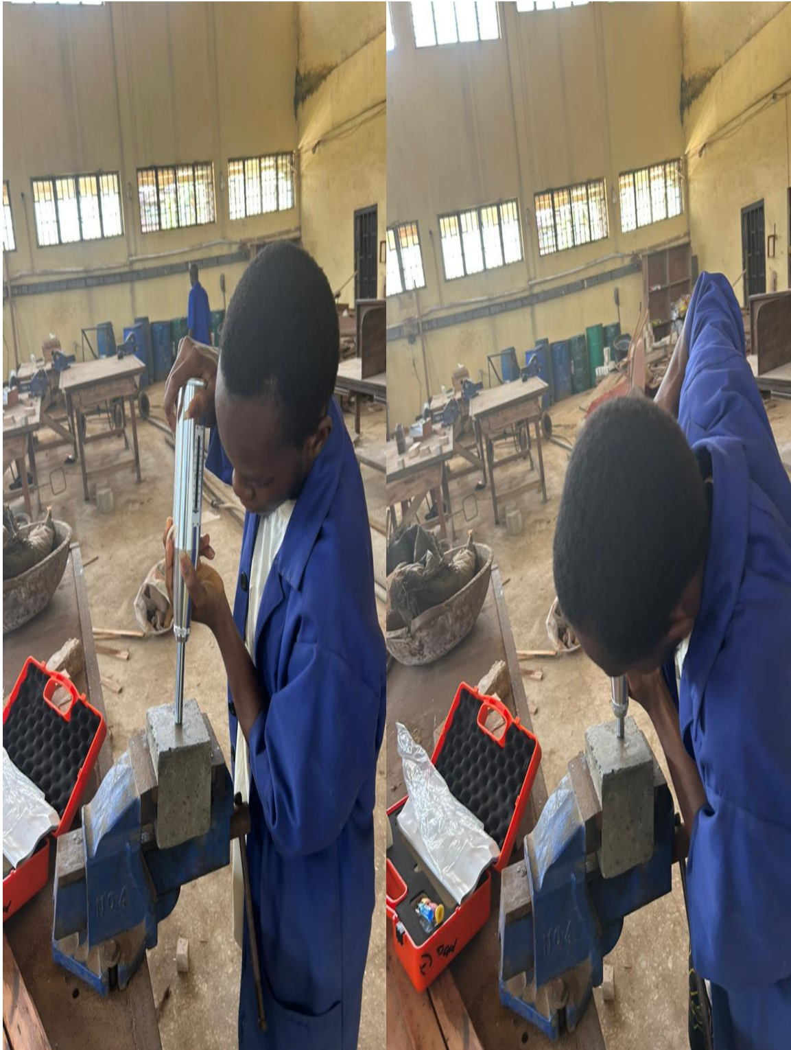
Plate 10: rebound hammer test (non-destructive test)
