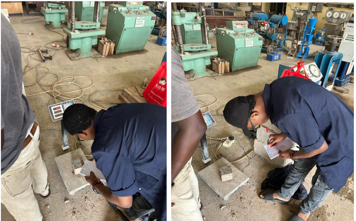
Figure A-2: Weighing the concrete cubes
