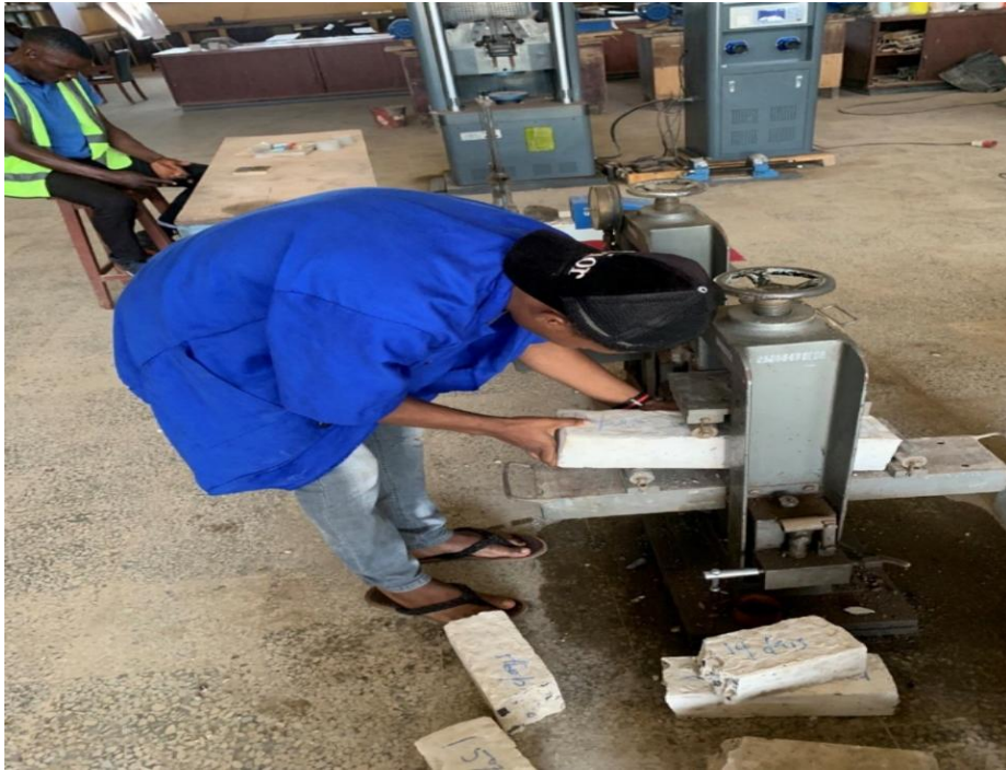
Figure A-3: Performing Flexural Test
