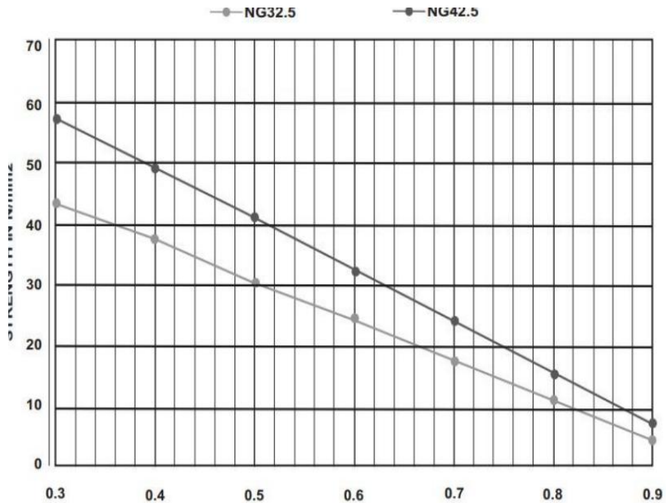
Figure 3.1: Strength versus Water/Cement Ratio for Nigerian Cements
