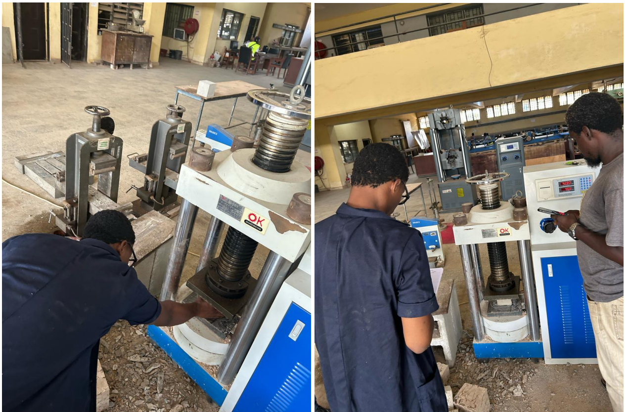
Figure A-4: Performing Compressive Strength Test
