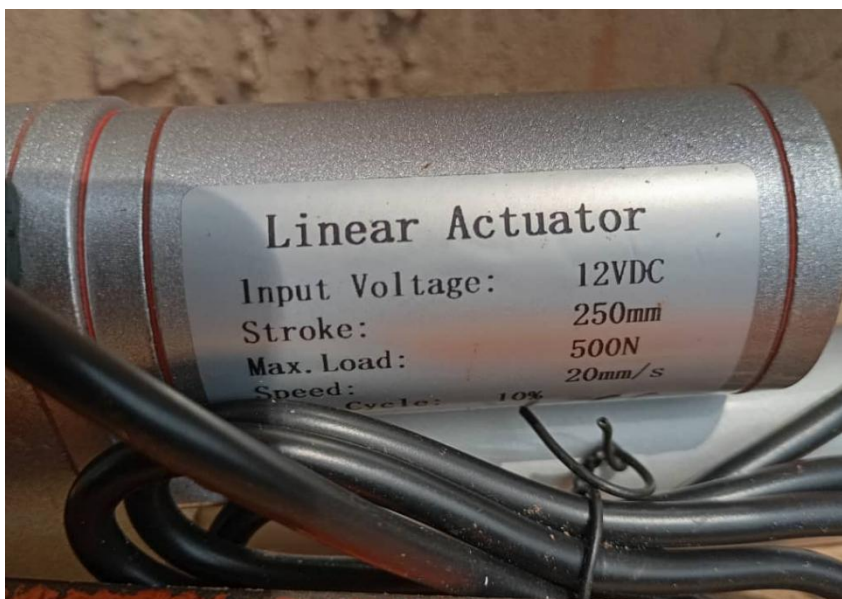
Fig. 3.15: Linear Actuator for Compaction
