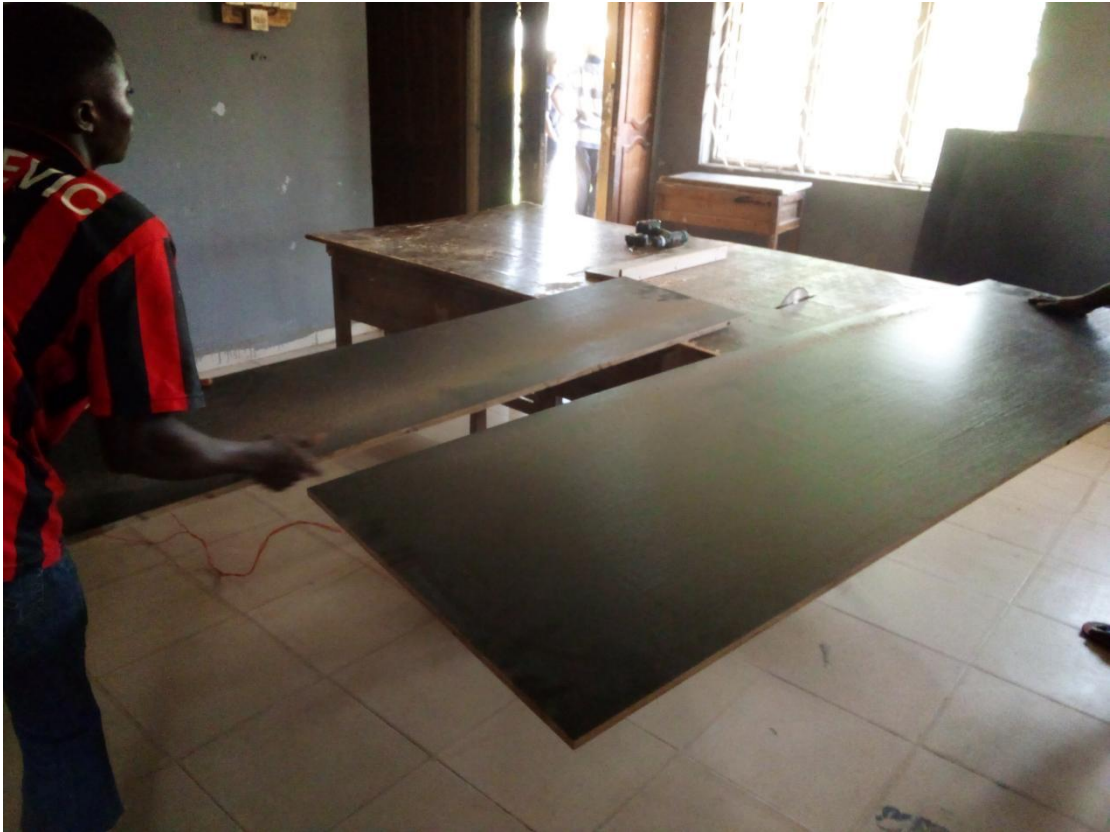
Fig. 5 Cutting of the hdf board to desirable size
