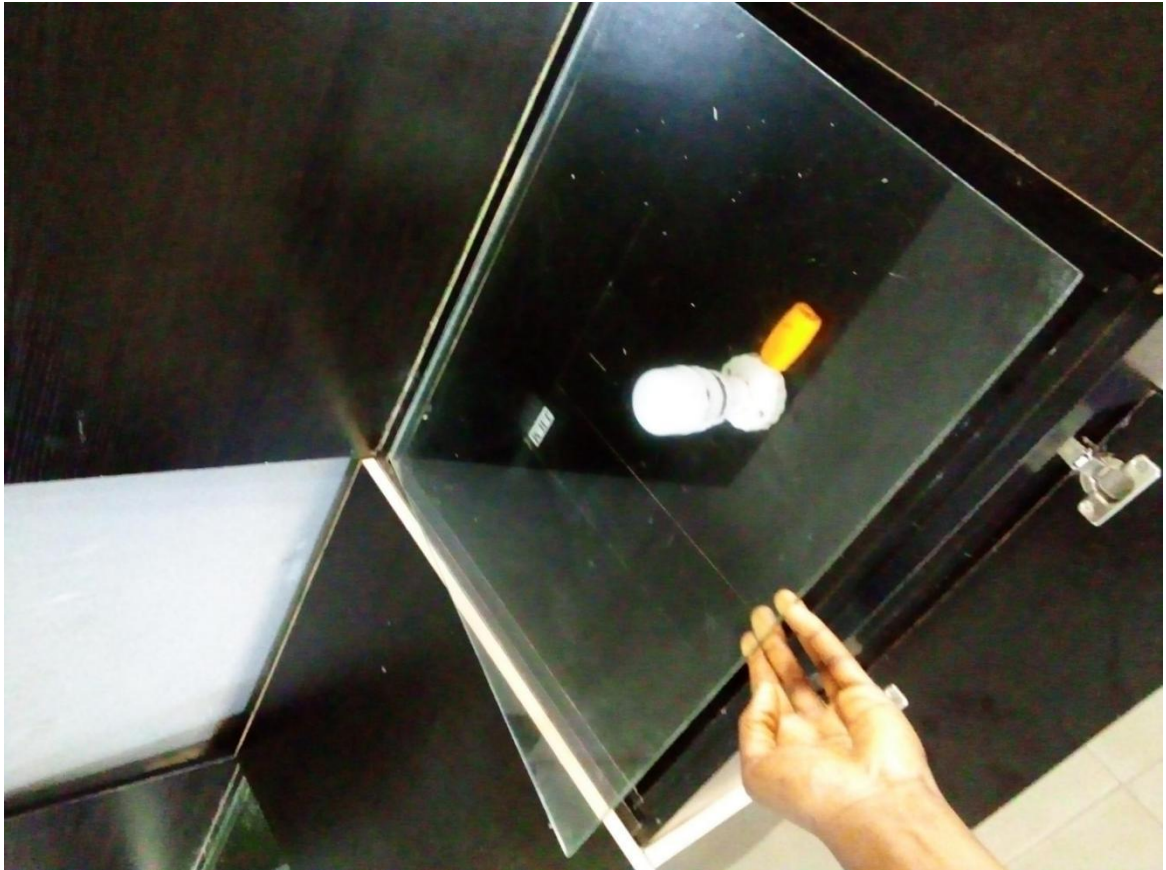
Fig.14 Fixing of glass in the light box
