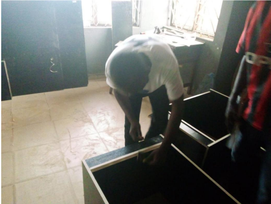
Fig.8 Using elephant gum to attach edge tape at the edges of the cut board to give it finishing look.
