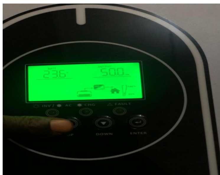
Figure 4.15: FREQUENCY OF OUTPUT VOLTAGE FOR LOCAL INVERTER
