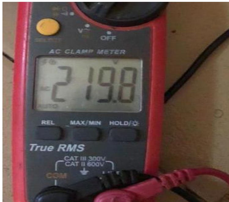
Figure 4.13: OUTPUT VOLTAGE TEST FOR LOCAL INVERTER
