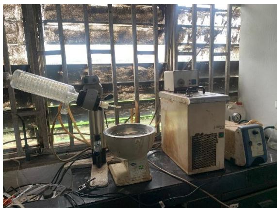
Fig 3.5 Image showing the rotavap used
