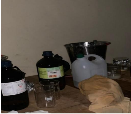
Fig 3.1 Image showing some materials used (sieve cloth, distilled water, absolute ethanol, stainless steel container, beakers, aluminium foil).
