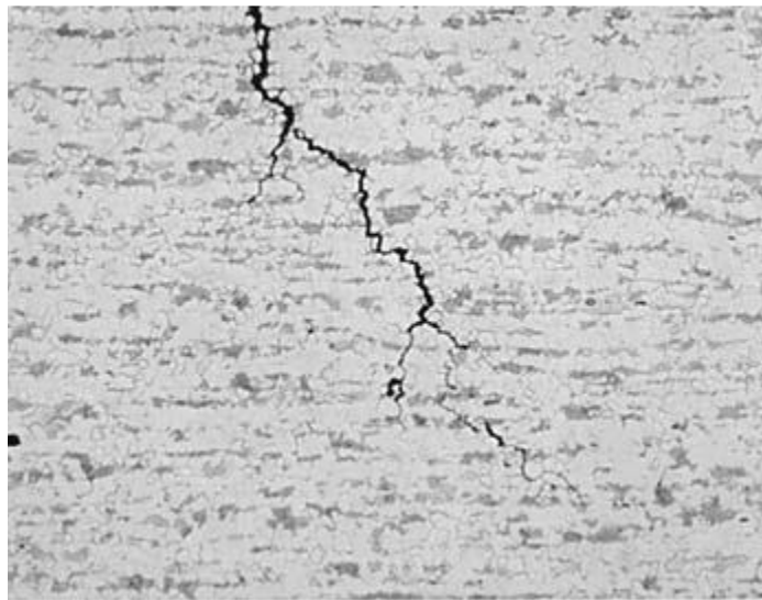
Figure 2.9: Intergranular high-pH stress-corrosion crack inline pipe steel. Nital etchant. Original magnification:400 X (Beavers et al., 2006)
