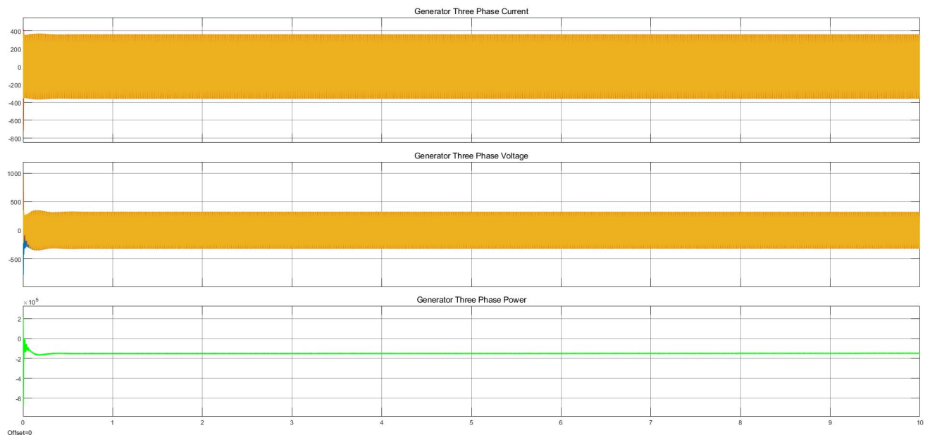
Figure 4.1: Graph showing the current, voltage, and power supplied to the 150KW load.
