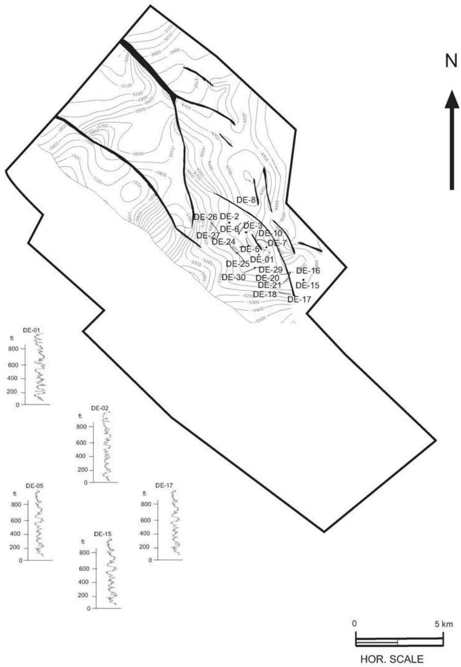
Figure 19. Structure map of intra-sequence 2. Log patterns show an overall aggrading to prograding pattern.
