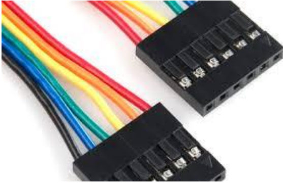
Figure 3.5a, Six-position crimp-type cable. Each wire is individually stripped, a connector crimped to it, and then the connectors are inserted into the plastic frame
