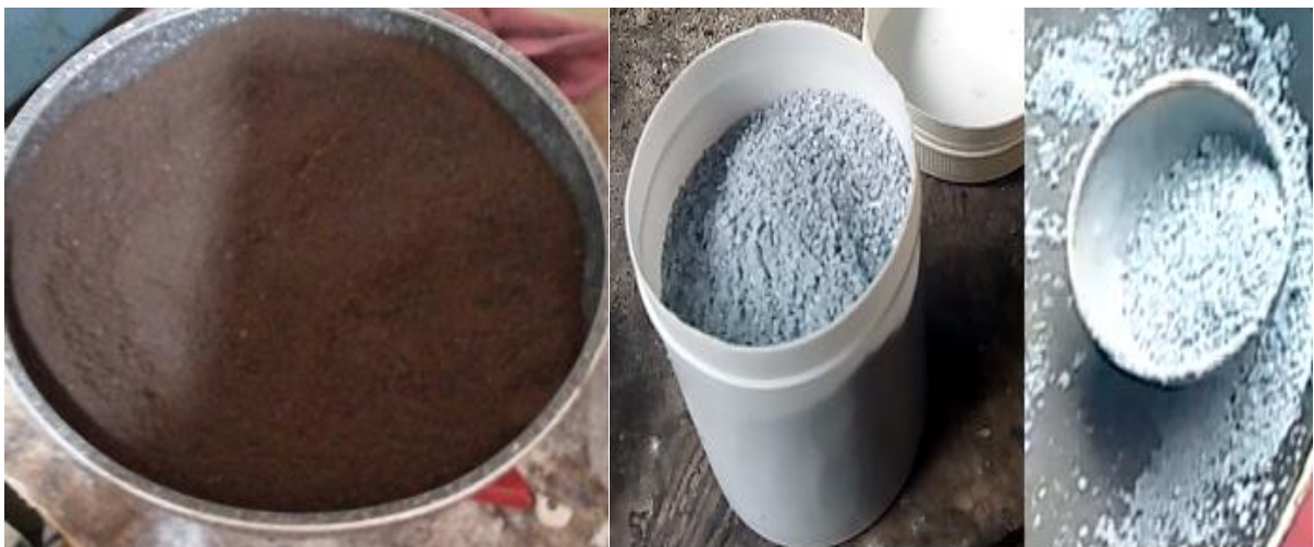
Figure 4.1(a) Uncalcined ripe plantain peel (brown) (b) Calcined ripe plantain peels (blue)
