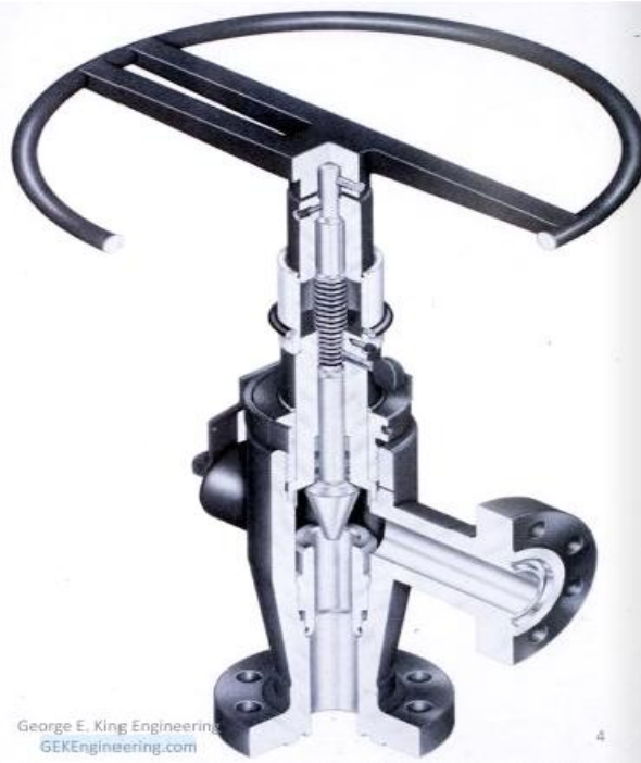
Figure 2.2: Variable Orifice Size (External Adjustment)
