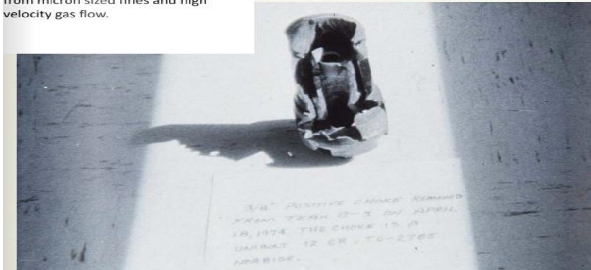
Figure 2.15: Erosion in a positive choke bean
