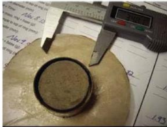
Figure 2.3. Digital micrometer used for the measurement of the diameter and thickness of shrinkage specimens. (D.G. Fredlund and S.L. Houston, 2013)
