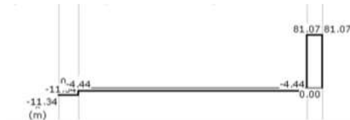
Figure 3.5: Horizontal shear force diagram for shaft I
