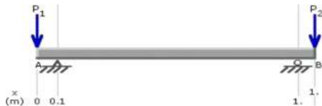
Figure 3.1: Vertical loading configuration for shaft I
