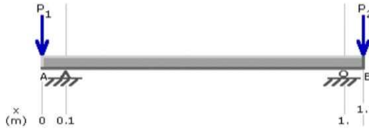
Figure 3.4: Horizontal loading configuration for shaft I
