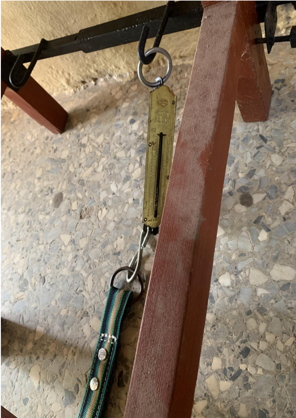
Figure 6: Image of the improvised leg dynamometer attached to a wooden chair
