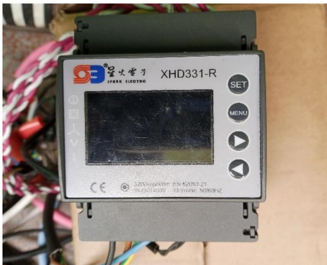
Figure 2.7: Spark Electro XHD331-R Smart Meter
