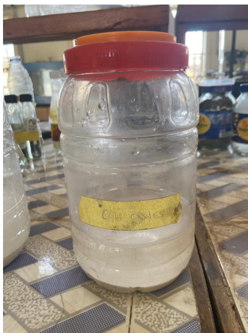
Plate 3.2: Calcinated cow bones been treated with Potassium hydroxide in an airtight container
