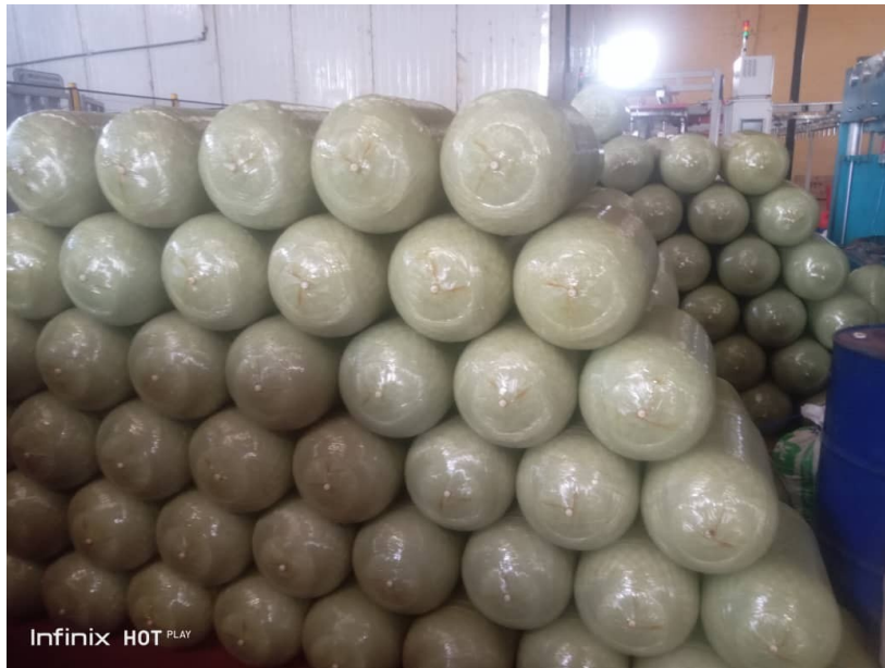
Figure 3.19: Composite cylinder with epoxy resin and hardener after curing
