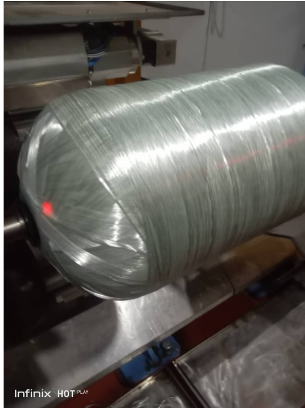
Figure 3.18: Composite cylinder with epoxy resin and hardener before curing
