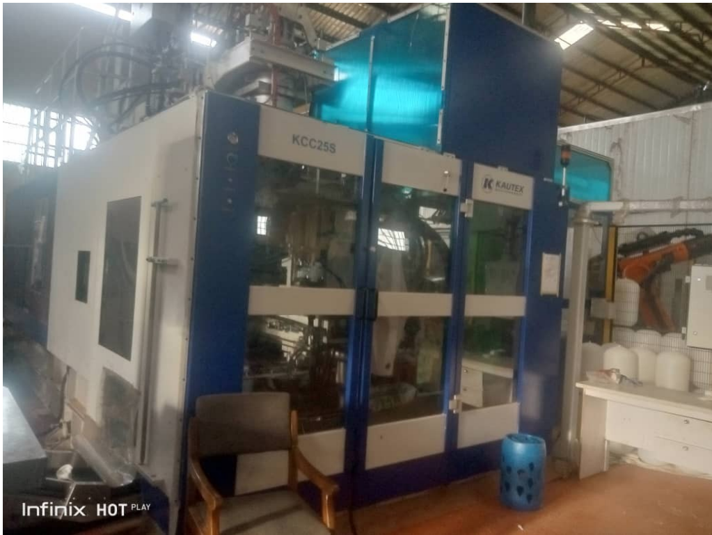
Figure 3.10: Blow Molding Machine
