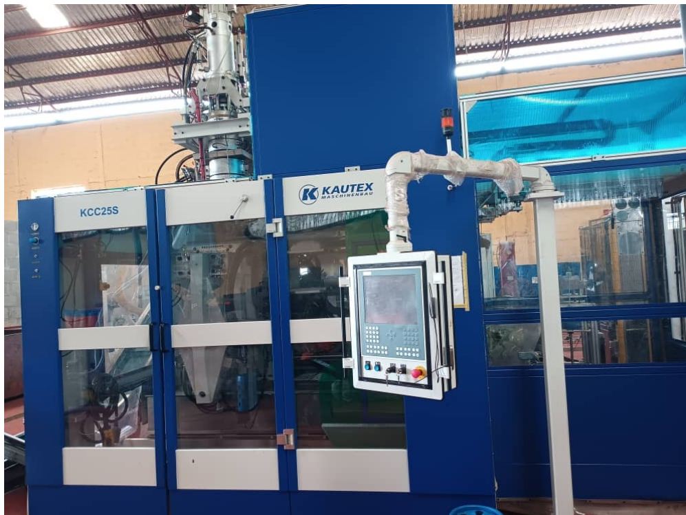
Figure 3.11: Blow Molding Machine
