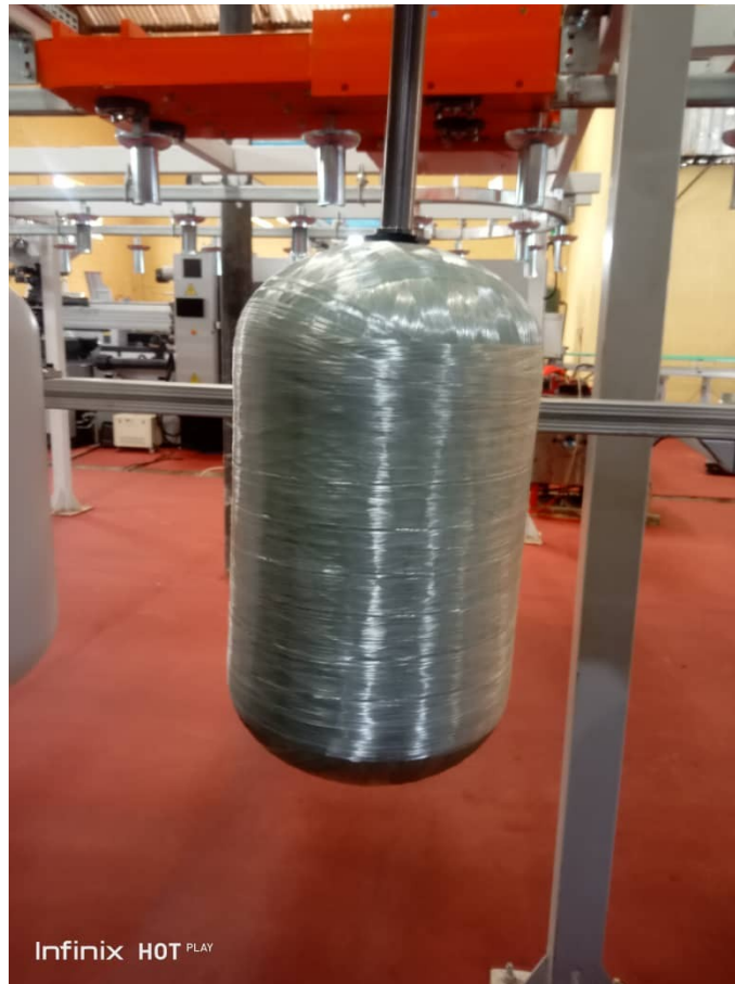
Figure 3.17: Type 4 composite cylinder with epoxy resin and hardener before curing
