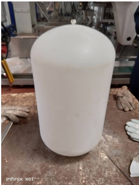
Figure 3.1: High Density PolyEthelene(HDPE) Polymer Liner
