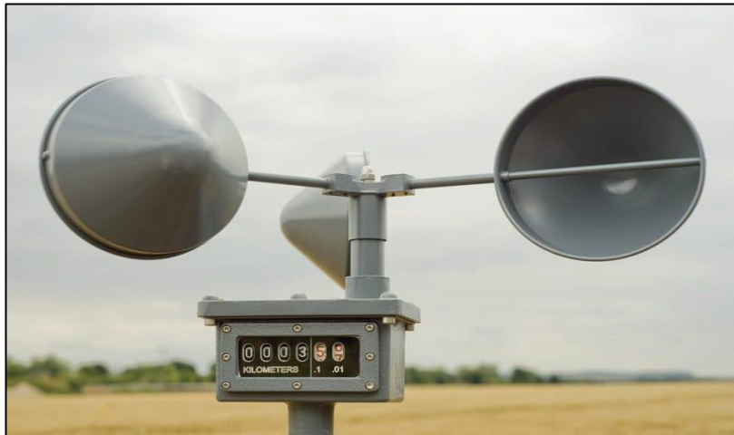
Fig 2.3c Mechanical Cup-counter anemometer
