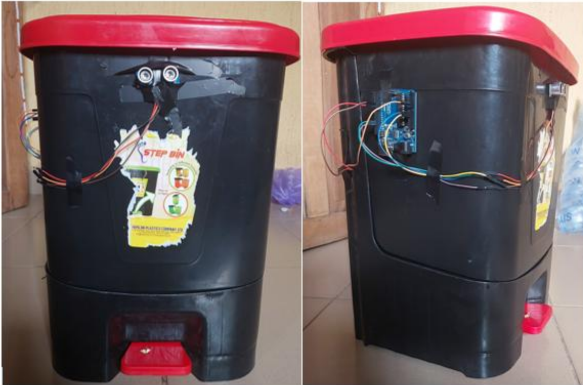
Figure 1: image of automated wastebin with microcontroller and sensor
