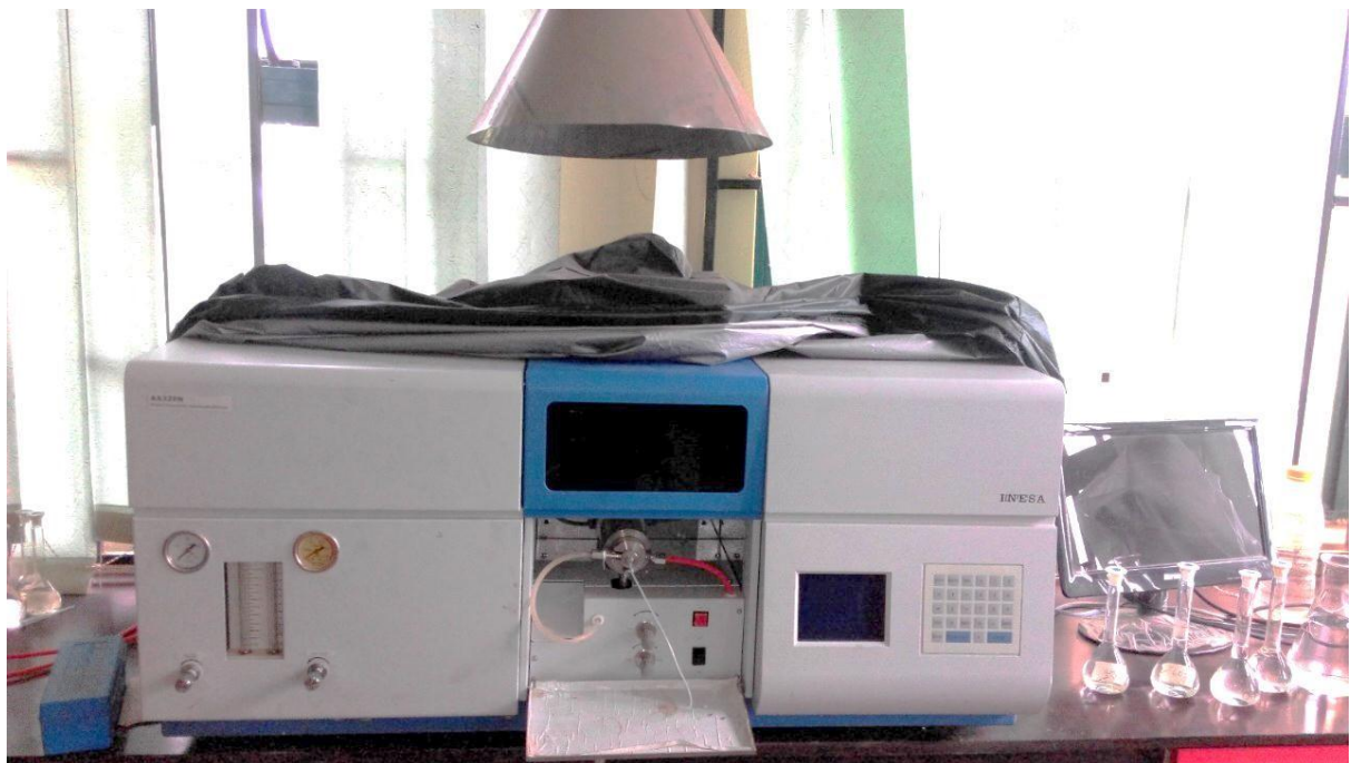
Fig 2: Atomic absorption spectrophotometer (Spectrophotometry and chromatography lab NCEE, Benin city.
