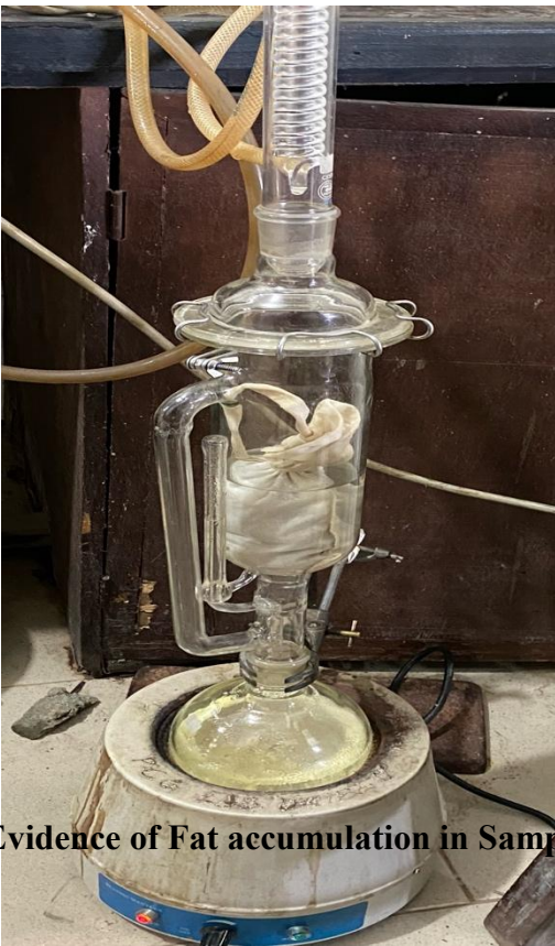
Soxhlet extraction set up
