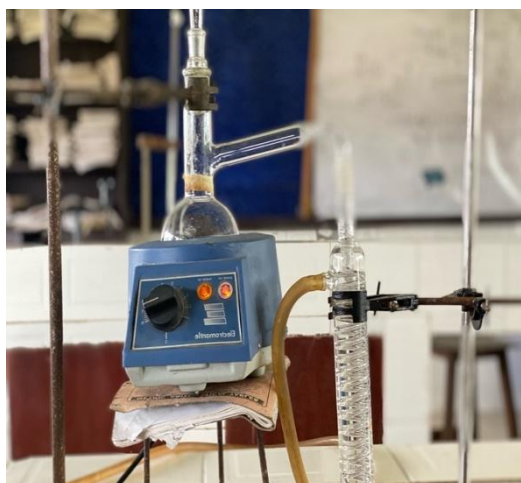
Kjeldahl distillation set up for protein determination and titration
