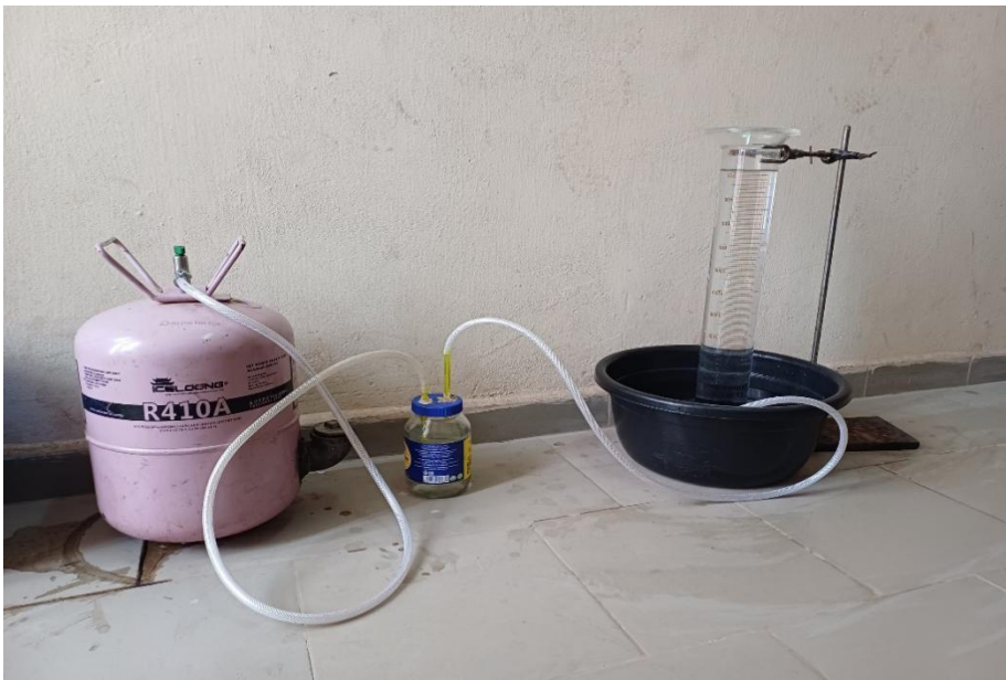
Plate 3.2: Experimental set-up for the Anaerobic digestion of Cow dung and Tiger nut waste
