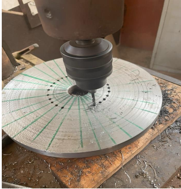
Plate 3.7: Drilling of the die plate
