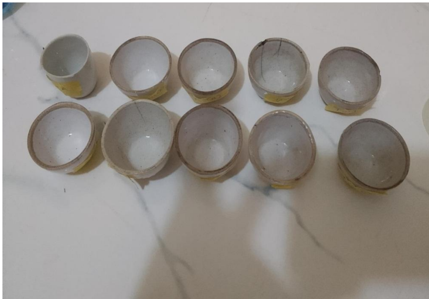
Plate 3.2: Evaporating dishes containing water samples collected from tap, Hand-dug well, and river sources for physicochemical analysis.
