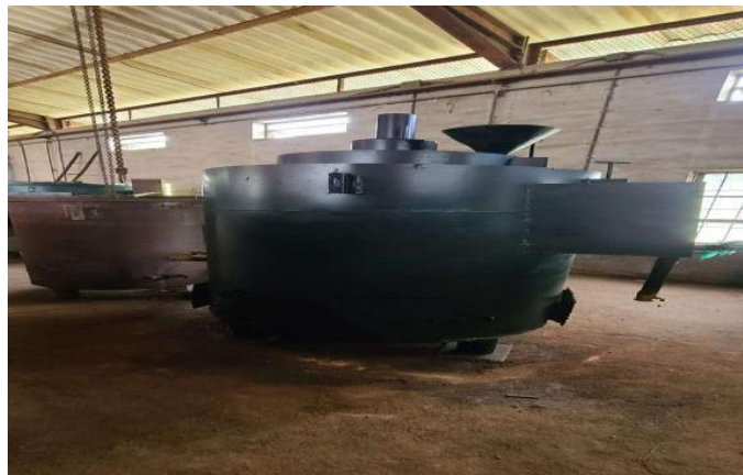
Figure 4.14: Clarifier used for separating palm oil from water and sludge during processing at NIFOR
