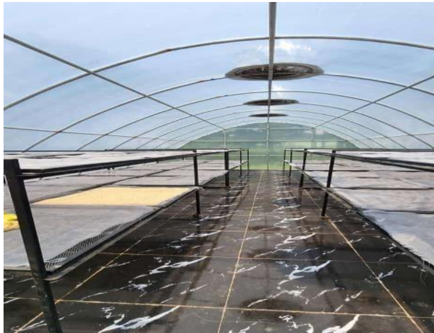
Figure 4.31: Modern solar dryer facility observed during fieldwork, used for hygienic and efficient preservation of vegetables and fruits.
