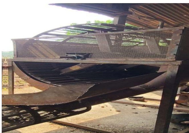
Figure 4.17: Full bunch stripper designed to detach fruitlets from palm fruit bunches.
