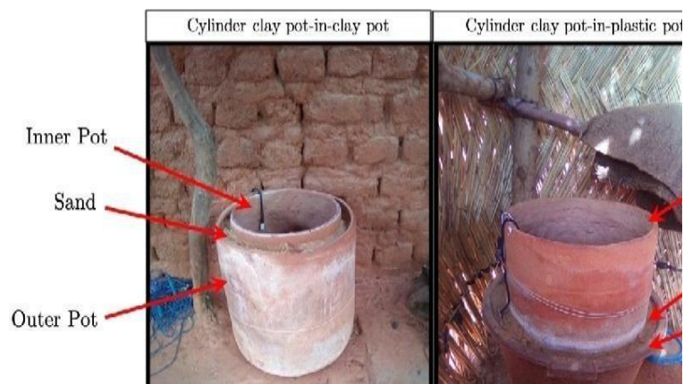
Figure 2.16: Pot-in-Pot Cooler (Source: https://www.semanticscholar.org/paper/A-heat-and-mass-transport-model-of-clay-pot-coolers-Rehman-McGarrigle/e0b0a4b433935961ed65119785131849682c48 )
