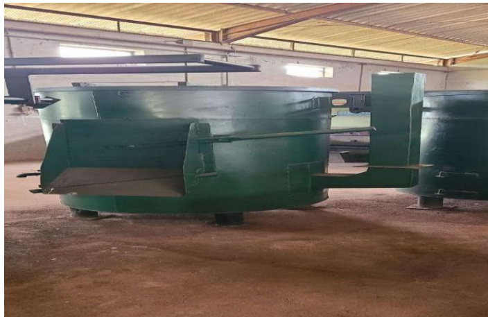
Figure 4.15: Sterilizer for steam-heating palm fruits to ease oil extraction.
