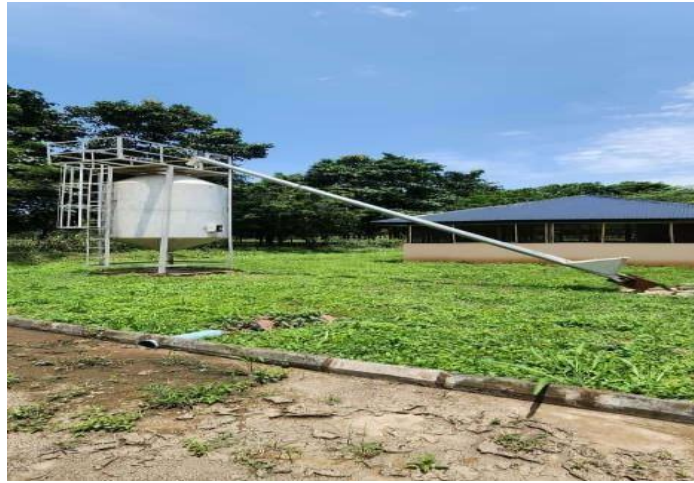
Figure 4.36: Modern silo facility observed during fieldwork, used for large-scale grain storage and protection against pests and moisture.
