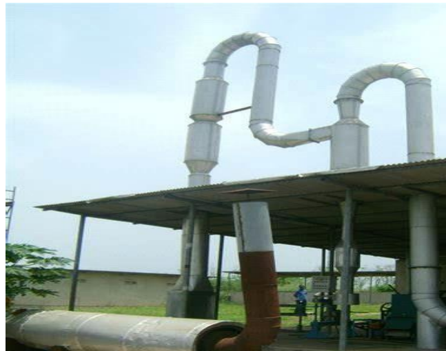
Figure 2.8: Mechanized drying of cassava using Flash Dryers (Source: https://th.bing.com/th/id/OIP.J6BI9Sah11F980gwJjC23wAAAA?rs=1 HYPERLINK)
