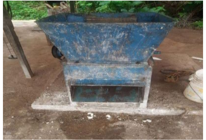
Figure 4.10 – 4.12: Locally fabricated cassava grinding machines used in small-scale garri production across Benin City.
