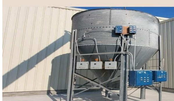
Figure 2.15: A galvanized steel silo used for large-scale grain storage. The structure provides a controlled, moisture-resistant environment that protects grains from pests and spoilage.
