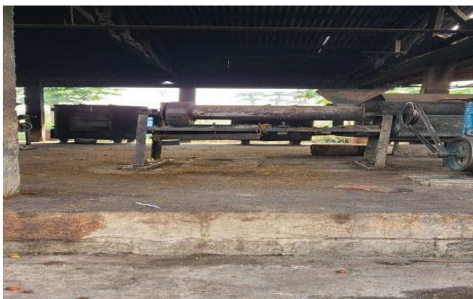
Figure 4.16: Digester screw press used to crush sterilized palm fruits and release oil.
