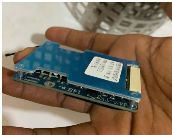
Figure 3.6: Battery Management System
