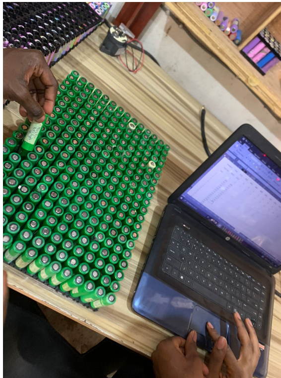
Figure 3.5: Module balancing in process
