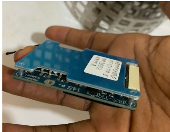
Figure 2.6: Battery Management System
