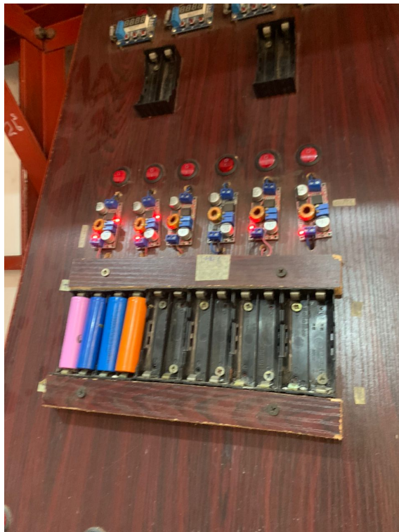
Figure 3.3: Charging is done for cells which are too low to be detected by the capacity tester
