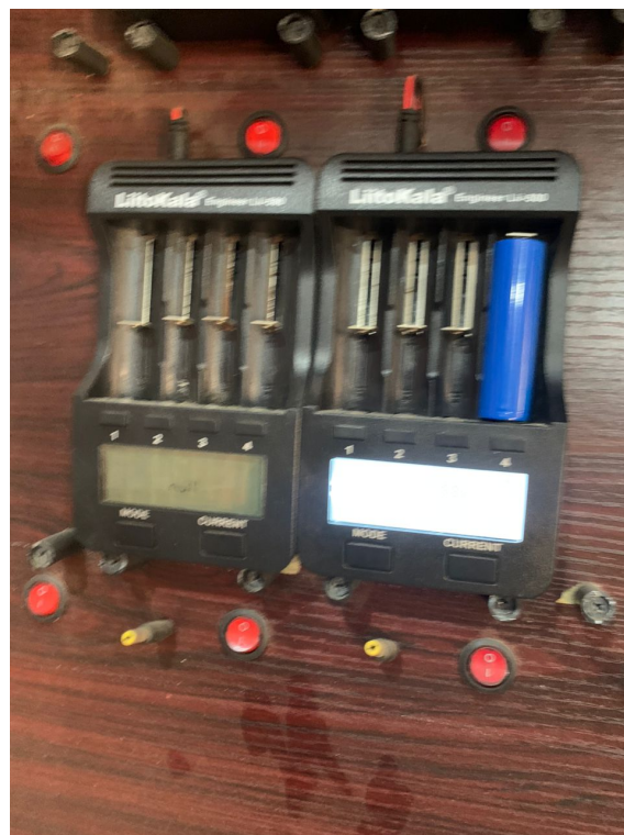
Figure 4.3: liito kala capacity testing machine capacity test
