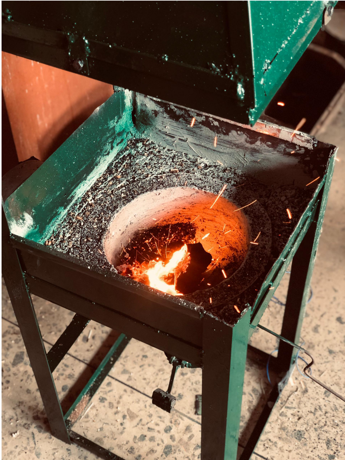
Plate 4.2 Firing test of the fabricated forge facility
