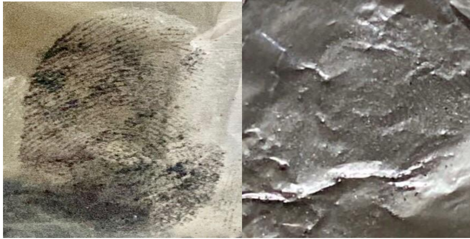
Fig 12: Images of latent fingerprint pattern on glass slides with powder from date palm seed latent fingerprint powder (a) and commercial latent fingerprint powder (b).
