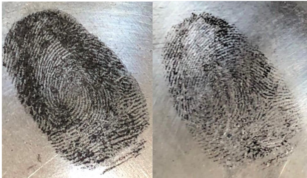
Fig 13: Images of latent fingerprint pattern on aluminium foil paper with powder from date palm seed latent fingerprint powder (a) and commercial latent fingerprint powder (b).
