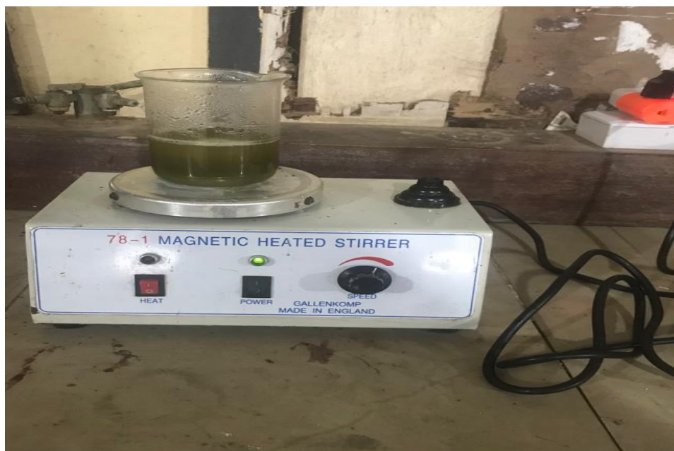
Fig 8: Magnetic stirring of date palm seed ash with HCl
