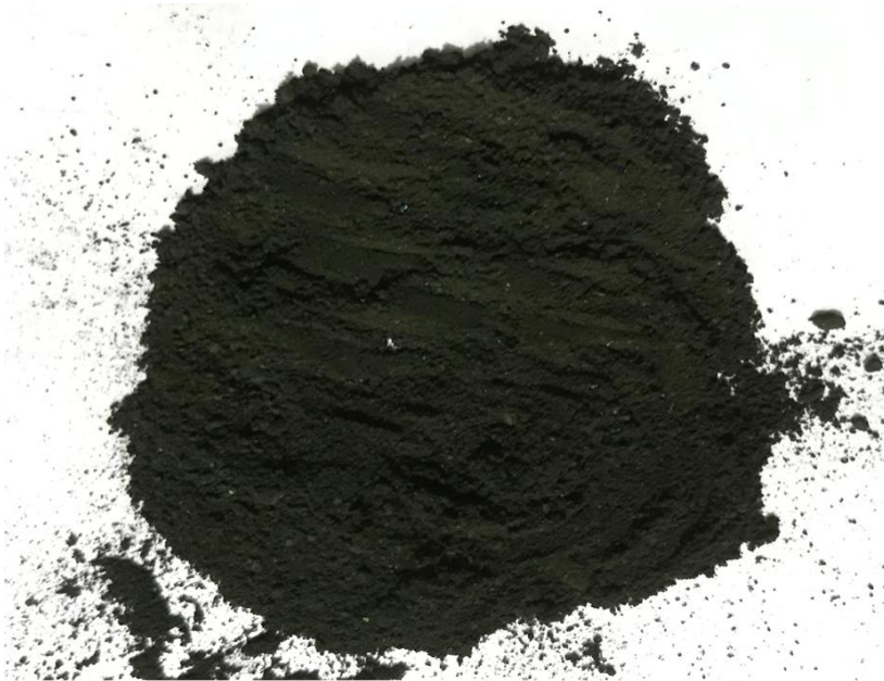
Fig 10: Latent fingerprint powder with methylene blue as dye
