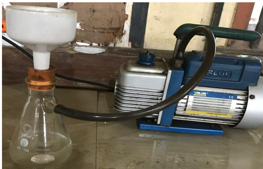
Fig 7: Filtration of solution using vacuum pump
