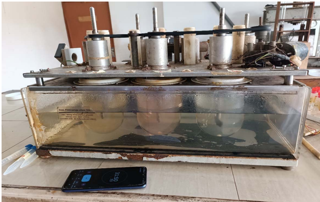
Rotating Paddle dissolution apparatus (USP Type 11) and digital stop clock
