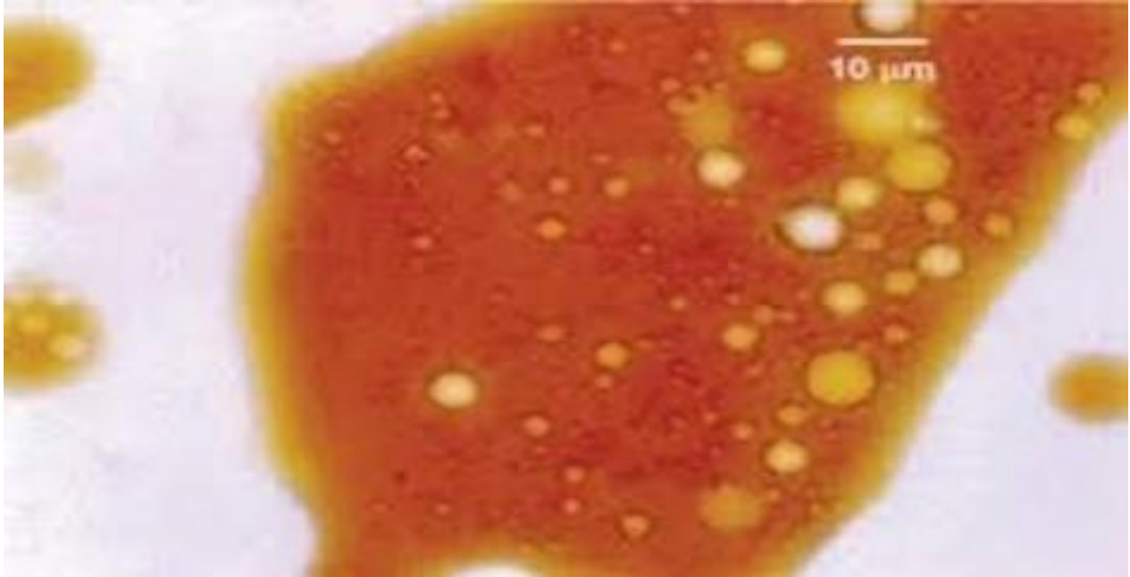
Figure 2. 2 photomicrograph of oil in water emulsion (kimray inc,2025)
