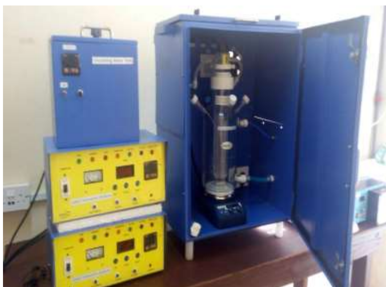
Fig 3.1 Multi-Lamps UV flow through photocatalytic reactor
