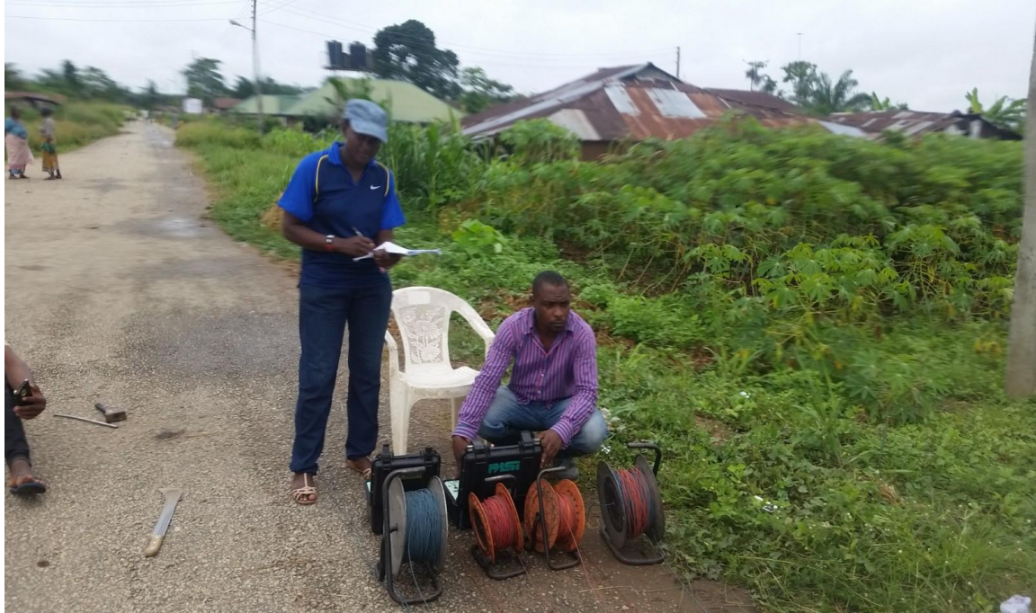
Plate 4: Recording the reading from the PASI Terremeter 16GL-N Model
