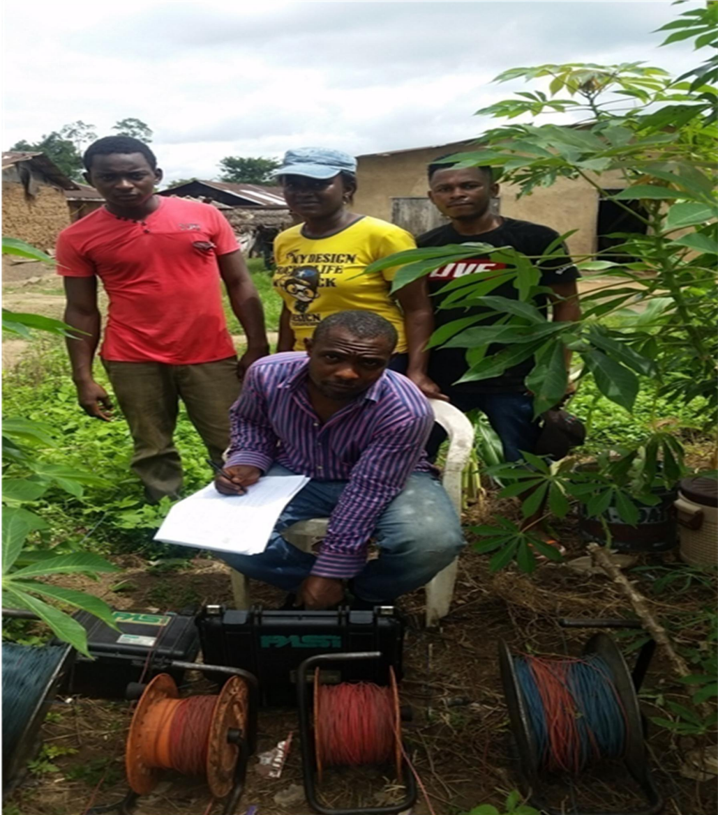
Plate 8: Taking of reading with the PASI Terremeter
