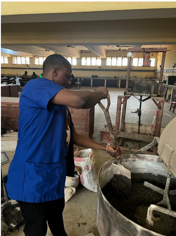
Plate 2: Mixing process for the concrete
