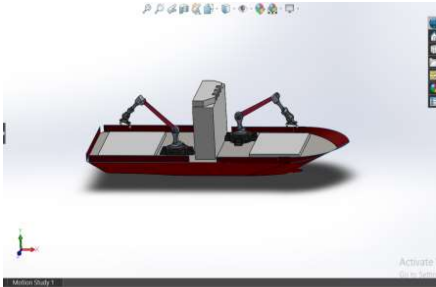
Figure 25 Dual Fore and Aft Crane Placement
