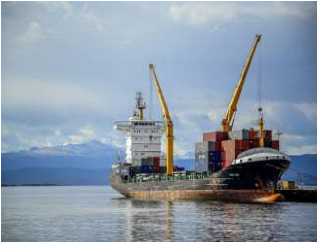
Figure 6 Swivel crane mounted on a vessel.
