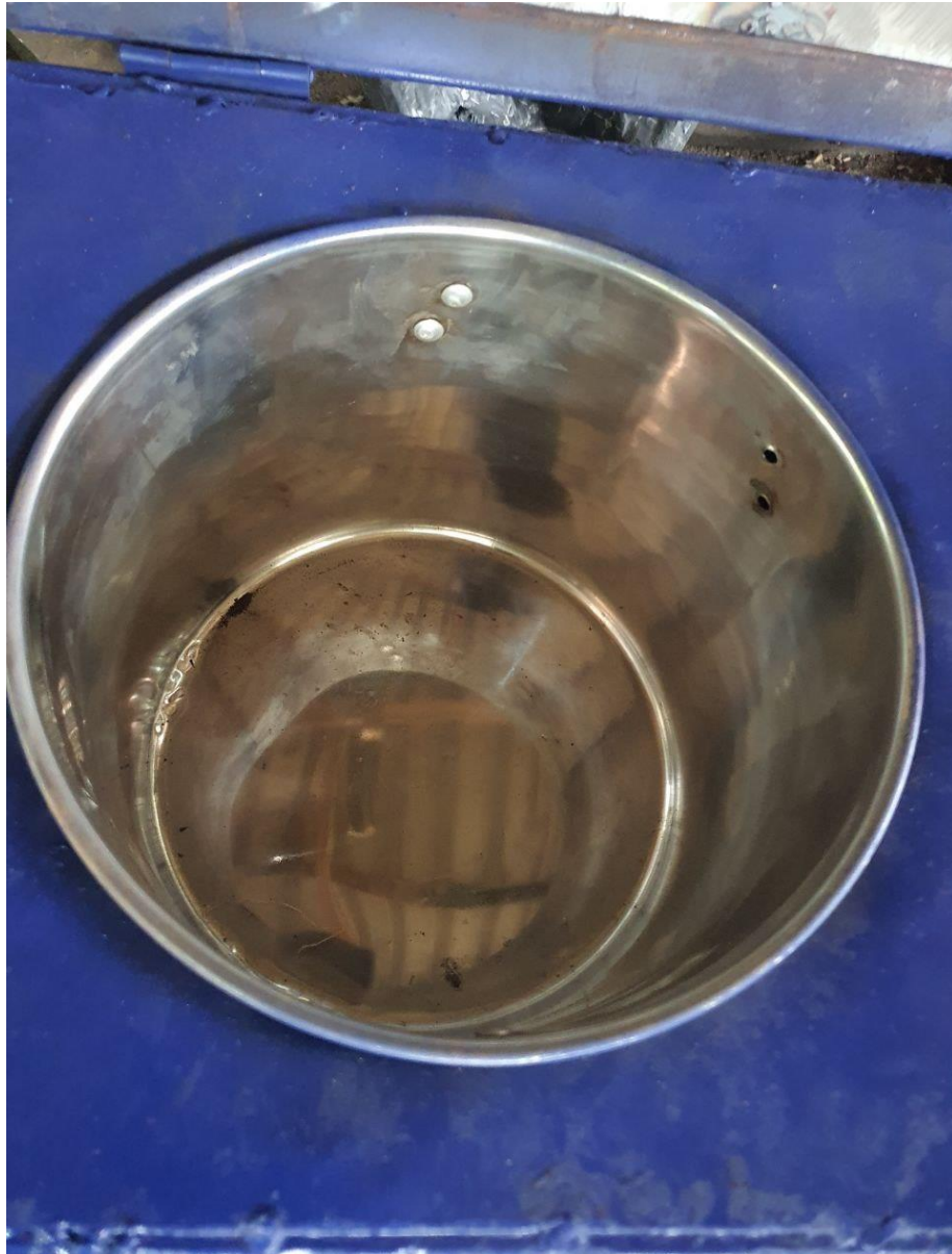
Fig. 3.17: The internal compartment of the system made of stainless steel
