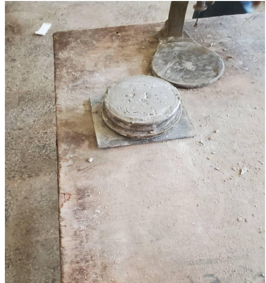
Fig 3.9: Determination of The Consistency and Setting Time of Cement Using Vicat Apparatus
