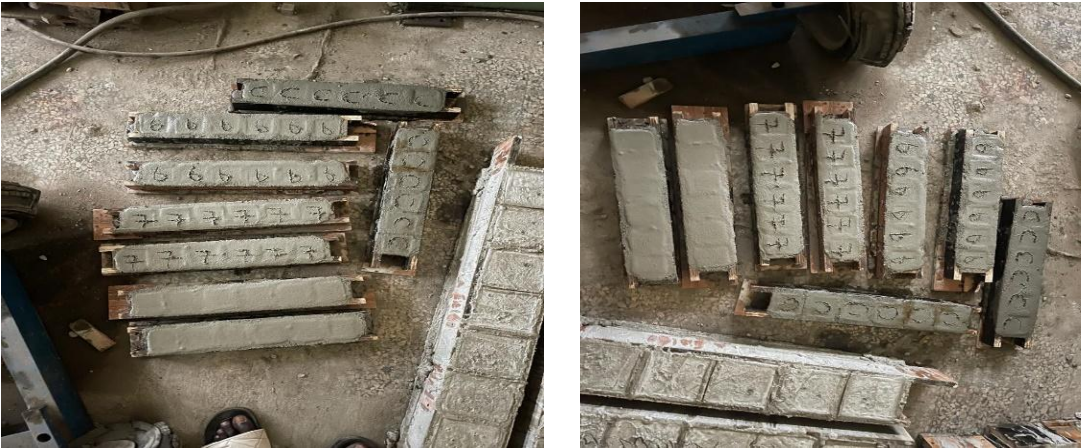
Fig 3.6: Identification of mortar cubes in mould
