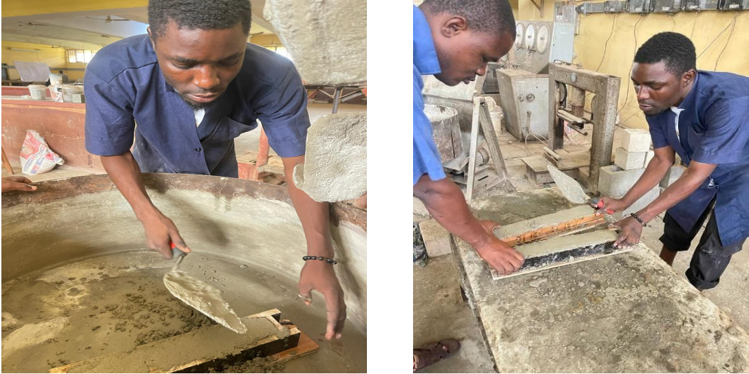
Fig 3.5: Casting and Compaction of mortar cubes
