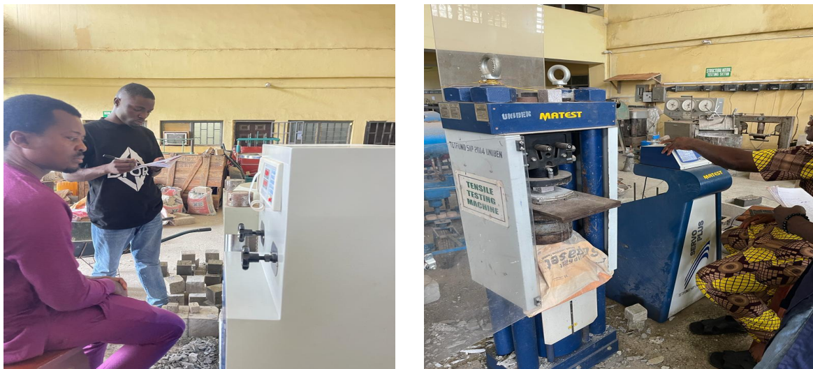
Fig 3.8: Crushing of Mortar Cubes on a Digital Compressive
