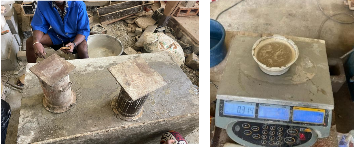
Fig 3.11: Determination of The Bleeding of Concrete for The Control and Replacement
