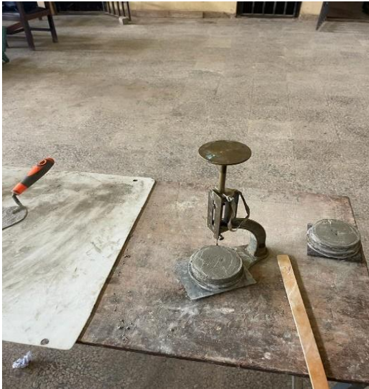
Fig 3.9: Determination of The Consistency and Setting Time of Cement Using Vicat Apparatus
