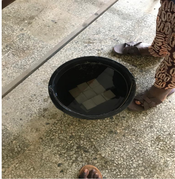
Fig 3.10: Immersion of The Control and Replacement Cube for Water Absorption Test
